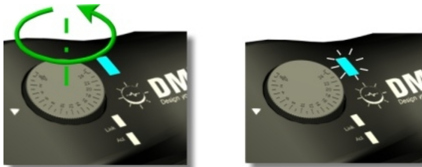
Figure 12: DMX port selection as input
