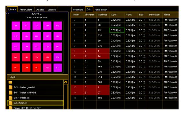
This view offers an overview about all used LED panels. All values can be edited directly in the grid. Selected panels are displayed bold. Patch collisions are indicated and marked red.
