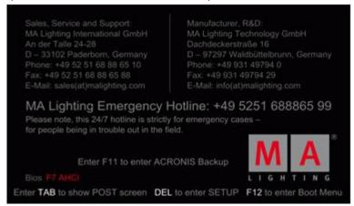
Stood in January 2010, you have to force the graphic card to do 800x600 to work correct with the internal screen on a VPU Plus. Otherwise you will see graphical artefacts and not readable fonts!
