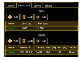
**Area/Output:** The general output of MA VPU is done now via the Ethernet protocol Artnet instead of the graphic card of the PC. Therefore the physical dimensions of the LED matrix (Area) and the number of pixels (Output) can be set:
