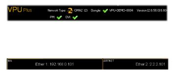
The headline informs about the network type and VPU software version, the session ID and name of the show. Also the active outputs Pixelmapper and DVI are shown.
