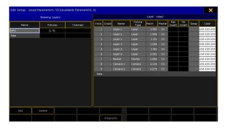
A layer in MA VPU is analog to a Fixture in the grandMA desk.
