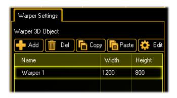
In the 'Warper Settings' you can define a Warper object. It is handled by the VPU like the other 3D Objects but it only has 2 dimensions X and Y.
