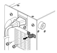
2. As shown in the figure, clamp the AC power cord with the AC Cord Clamp, and secure with the screws (2) removed in Step 1.
