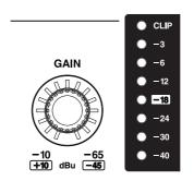
If the signal level exceeds 0 dB, the CLIP indicators on the LED input meter and signal status indicators will light and distortion will occur. For the best audio quality, set the preamp gain so the meter reads between -18 and -3 dB on the input signal's loudest peaks.
