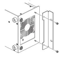
3-2. The bracket for the right side should be fitted as shown below and fixed with four screws (two screws that were removed in step 2, plus the two screws included in the package).
