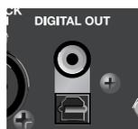
These jacks output a consumer format (IEC-60958 compliant) digital audio signal. Two types are provided: coaxial and optical. The same digital audio signal is output from both jacks. By default, MONITOR L/R is patched to these jacks.
