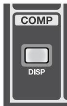
In this area you can operate the compressor that is provided on CH1–48 and the limiter that is provided on AUX1–16, MTX 1–8, and MAIN L/R/C.
