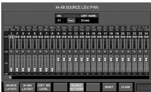
This shows the sources arranged in order of their number (the order in the M-480's REAC B output patchbay).
