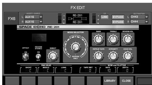
This is a delay that models the Roland RE-201 Space Echo. The original was mono-in, mono-out, but this modeling adds PAN HEAD SHORT/MIDDLE/LONG settings and a REVERB STEREO Sw, allowing you to use it as a mono-in, stereo-out effect.
