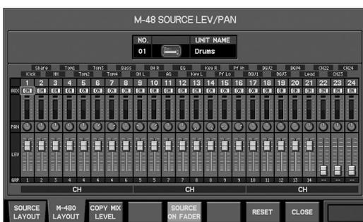
This shows the sources as they are seen from the M-480's fader module section. This display will change according to the M-480's fader layer.
