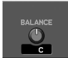
This adjusts the left/right output balance sent from MAIN L/R or stereo-linked AUX/MTX in a range of L63–R63.
