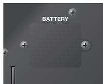
This slot contains a lithium battery that maintains the M-480's clock function and preserves the mixer settings.
