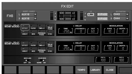
This is a delay that models the Roland SDE-3000 digital delay. The original unit was mono-in, mono-out, but this modeling provides a dual-mono configuration with two such units in parallel. The MOD LINK Sw allows you to use this as a stereo-in, stereo-out unit.
