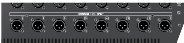
These are balanced XLR-3-32 male output jacks for outputting analog audio signals. By default, AUX OUT 1–8, MONITOR L/R are patched to them.
