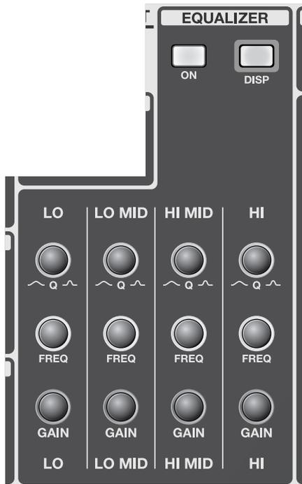
In this area you can operate the 4-band EQ that is provided on CH1–48, AUX1–16, MTX 1–8, and MAIN L/R/C.
