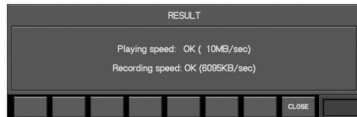
A "now processing" message will appear, and the USB memory will be tested. When the test is completed, the results will be displayed.
