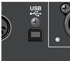
This USB connector can be connected to your PC to control the M-480 remotely.
