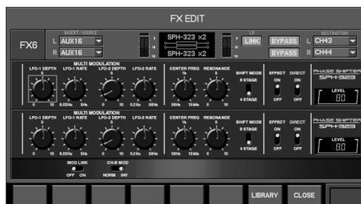
This is a phase shifter that models the Roland SPH-323 Phase Shifter. The original was mono-in, mono-out, but this modeling is a dual-mono design with two units in parallel. The MOD LINK Sw allows you to use this as a stereo-in, stereo-out effect.
