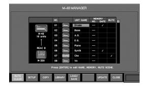
In the M-48 list, move the cursor to the NO. field of the desired M-48 and press [ENTER].
