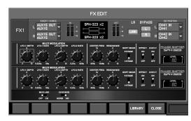
This is a phase shifter that models the Roland SPH-323 Phase Shifter. The original was mono-in, mono-out, but this modeling is a dualmono design with two units in parallel. The MOD LINK Sw allows you to use this as a stereo-in, stereo-out effect.
