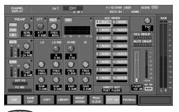
You can make adjustments in finer increments by holding down [SHIFT] while you operate the CHANNEL EDIT section's knobs or the value dial.
