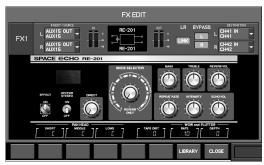
This is a delay that models the Roland RE-201 Space Echo. The original was mono-in, mono-out, but this modeling adds PAN HEAD SHORT/MIDDLE/LONG settings and a REVERB STEREO Sw, allowing you to use it as a mono-in, stereo-out effect. The RE-201 was a very popular product that was produced from 1974 to 1987.
