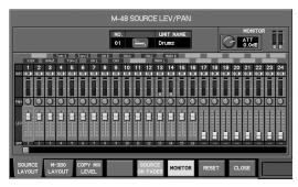
This shows the sources arranged in order of their number (the order in the M-380's REAC B output patchbay).
