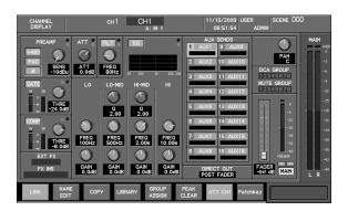
Even if you don't access the CHANNEL DISPLAY screen, the value of the currently-operated parameter is shown in the sub display area when you operate an dial in the CHANNEL EDIT section.
