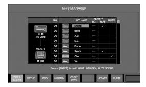
2. In the M-48 list, move the cursor to the MEMORY SAFE field of the desired M-48 and press [ENTER] to add a check mark. M-48 units with a check mark will not accept Store or Recall operations from the M-380.
