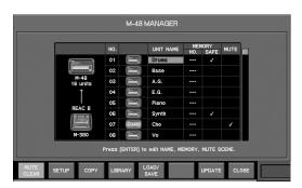
In the M-48 list, move the cursor to the desired copy-source M-48 unit, and press [F3 (COPY)].
