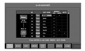
In the M-48 list, move the cursor to the MUTE field of the desired M-48 and press [ENTER] to add a check mark.
