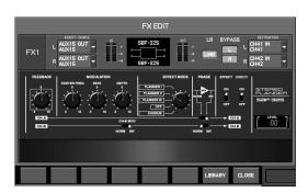
This is a stereo-in, stereo-out flanger that models the Roland SBF-325 Stereo Flanger.
