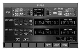
This is a delay that models the Roland SDE-3000 digital delay. The original unit was mono-in, mono-out, but this modeling provides a dual-mono configuration with two such units in parallel. The MOD LINK Sw allows you to use this as a stereo-in, stereo-out unit. The SDE-3000 was released in 1983, and was used in numerous recording studios and PA systems around the world.
