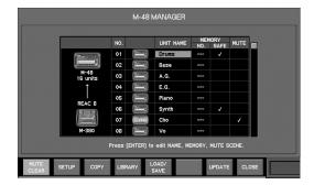
In the M-48 list, move the cursor to the UNIT NAME of the desired M-48 and press [ENTER].
