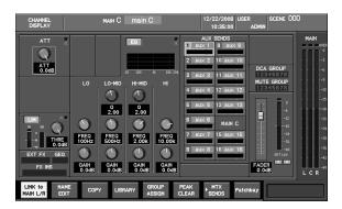
MAIN C has parameters that are equivalent to MAIN L/R. If you turn [F1 (LINK to MAIN L/R)] on, you'll be able to use the MAIN fader to control MAIN C while maintaining the fader balance between MAIN L/R and MAIN C.
